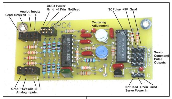
Analog input connector in upper left hand corner with 3 4 label:
