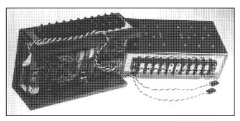
**OVERVIEW: RSFR** *DIRECTORs* perform speed and direction functions for a single motor of a Radio/Controlled vehicle. They're used for robots, boats and subs and two **RSFR**'s can be used
